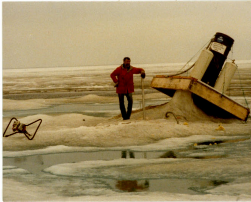
22. The EPC, as found on July 22 before removed for the season. Four guy wires through the ice kept the unit from toppling over. ( )
