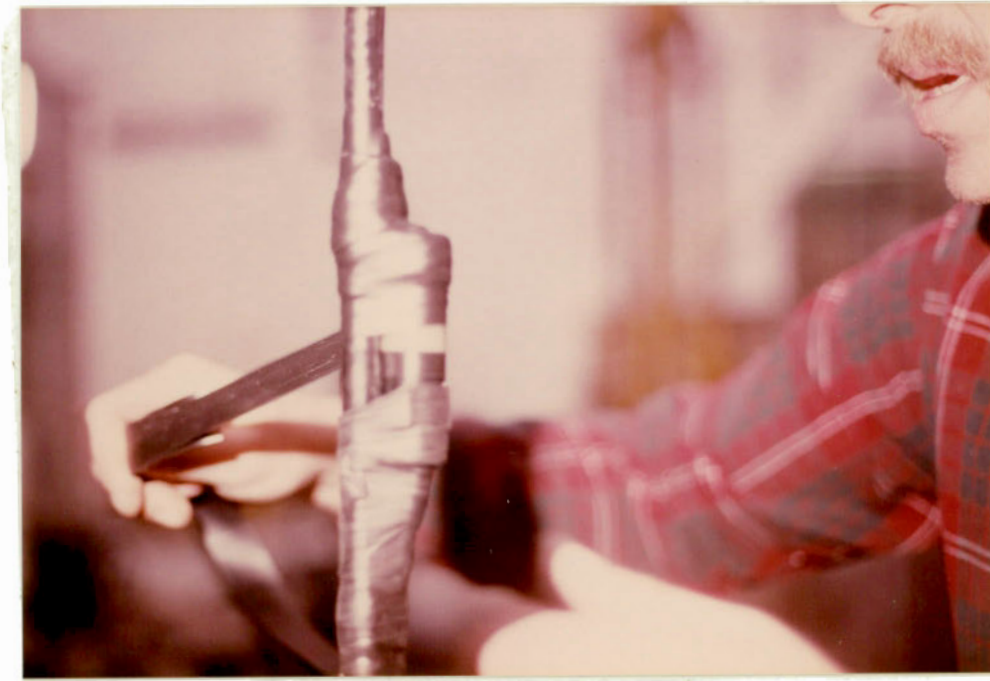
10. Nearing completion of streamlining with tape. (c15)
