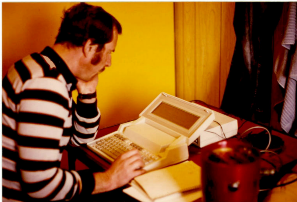
23. Mark Hill dumping data from the Mesotech model 612 surface recorder onto the HP110 computer. ( )
