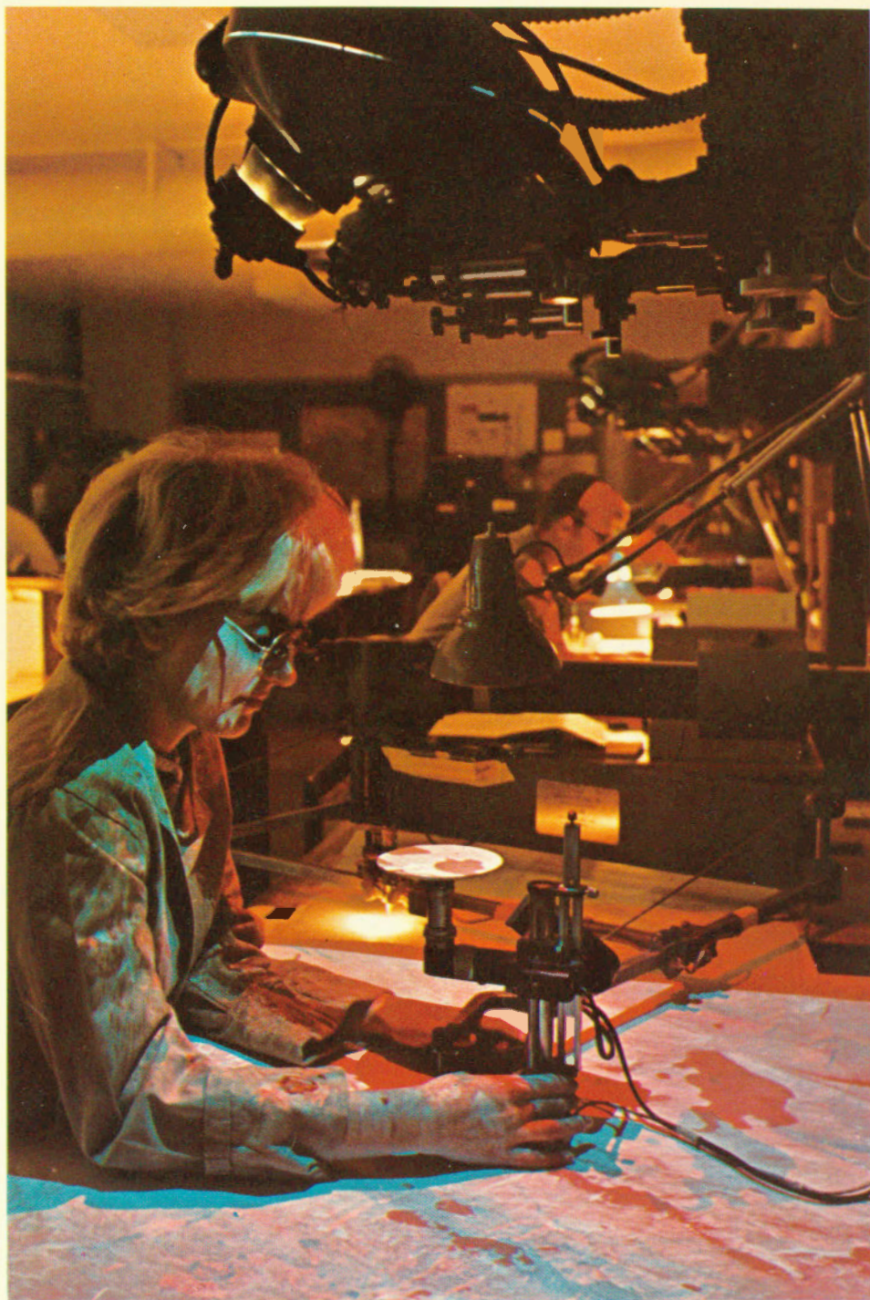
FIGURE 39. Operator compiling a map manuscript on a stereoscopic plotting instrument, aided by overhead projection of color images.
