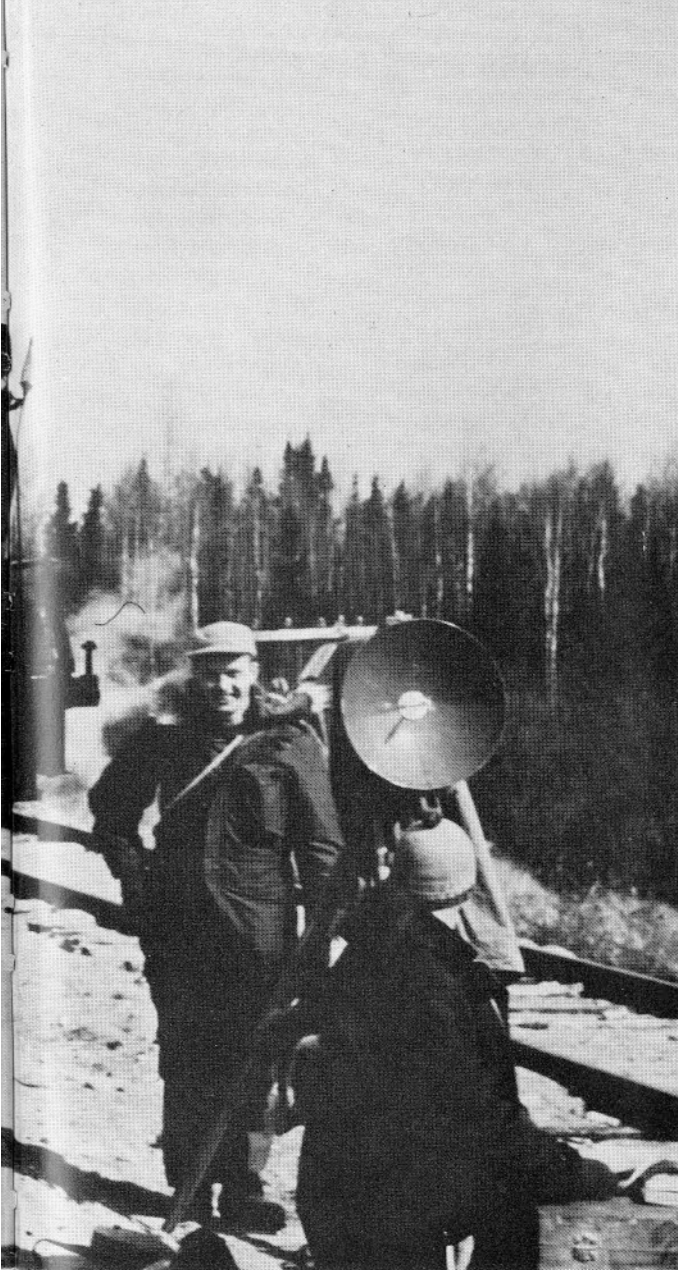
FIGURE 148 Army engineers on a tellurometer traverse, 1958, accommodated on a Hudson Bay Railway train.
