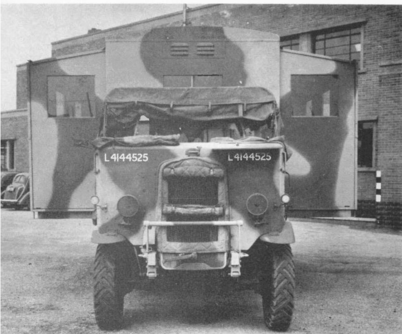
FIGURE 102 Leyland Retriever truck containing an army map press. Note extended sides to accommodate printing press.
