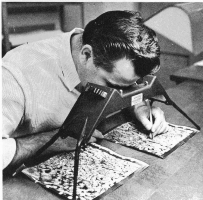
FIGURE 40 Map technician using stereoscope to assist identification of features on aerial photographs.
