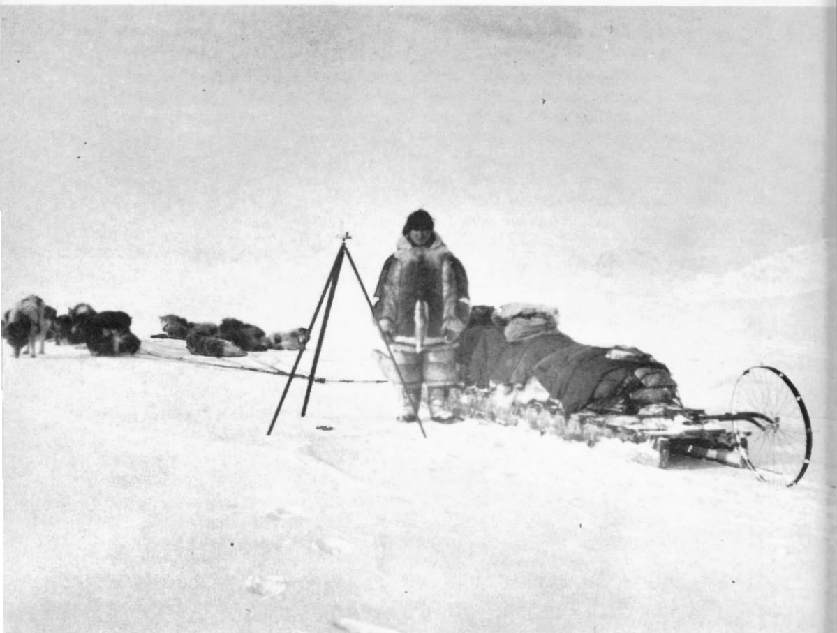
FIGURE 172. Winter survey work, using prismatic compass and odometer, Baffin Island, 1927.
