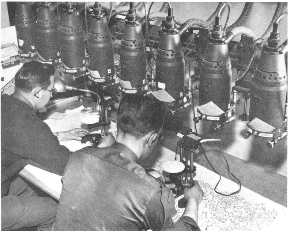
FIGURE 105. Army mappers using multiplex plotter for contouring.
