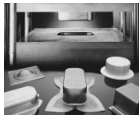
NRCan has expertise and equipment to investigate the formability of sheet steel and aluminum for applications such as vehicle bodies.
