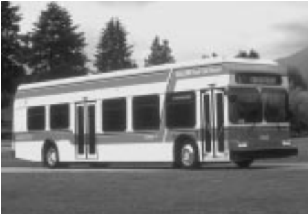
Developed by Ballard Power Systems, this zero-emission bus runs on hydrogen fuel cells.
