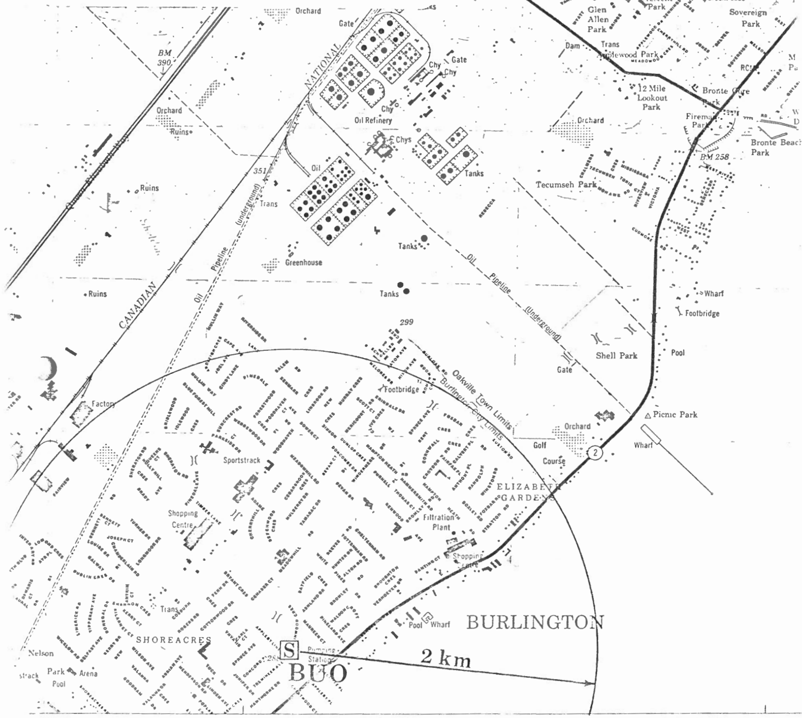
Figure 3. The area of the east end of Burlington, Ontario that has experienced the ground disturbances. The location of the seismograph station, BUO, is shown. The source of the disturbances almost certainly lies within 2 km of the station.
