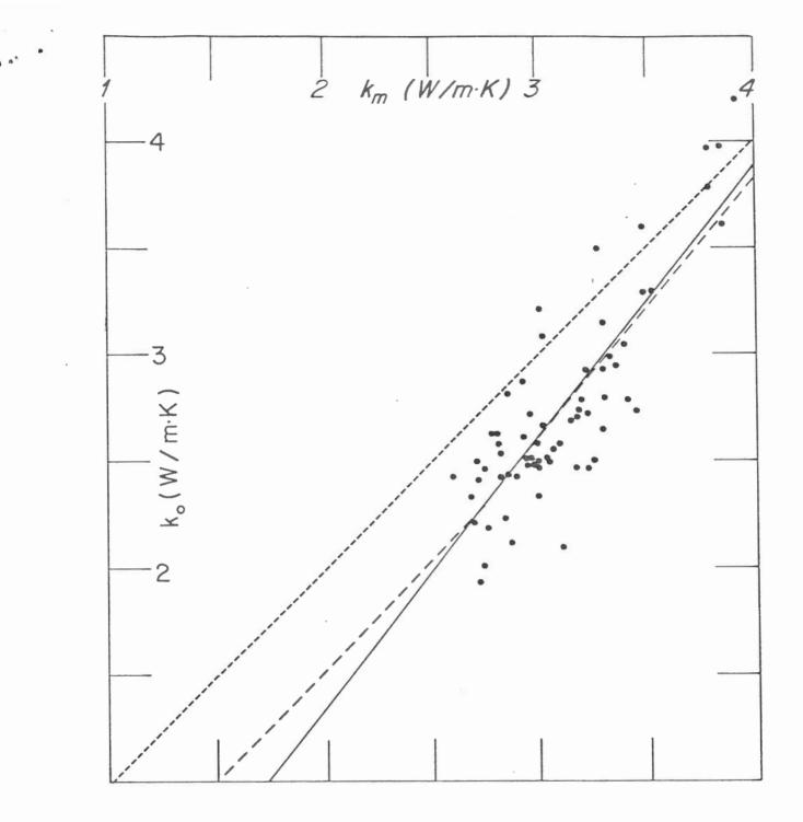
Fig. 1 Observed conductivity k<sub>o</sub> plotted against modelled conductivity
