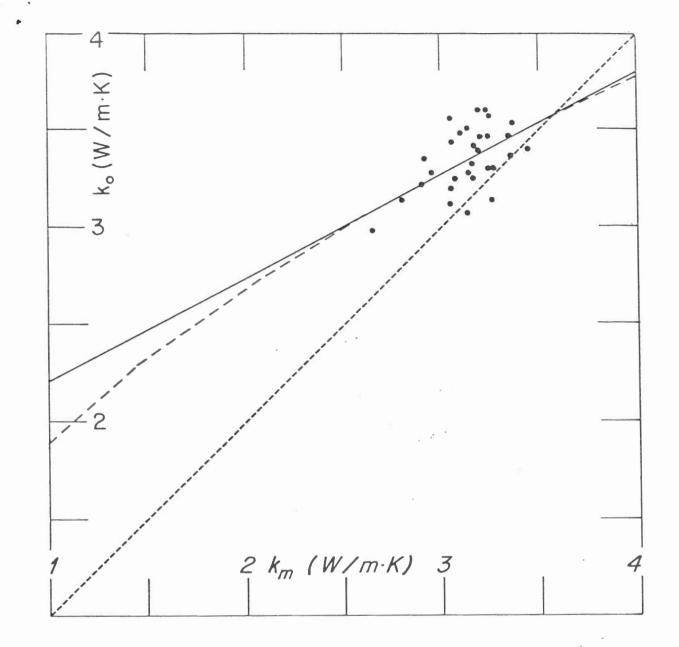
Fig. 2 Observed conductivity  $k_0$  plotted against modelled conductivity  $k_m$  for Whiteshell granites. Legend as for Fig. 1. Parameters are: a = 0.53, b = 1.68, R = 0.555.
