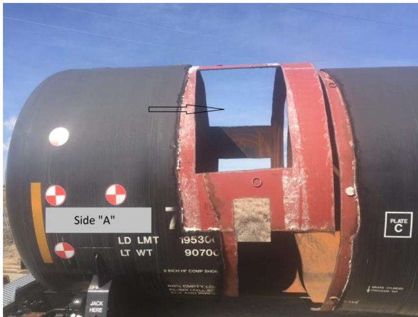
Figure 7: US Federal Railroad Administration impact-tested tank car, showing location of TC128B panel used in this work. Photo provided by Nolan Hanson of the Transportation Technology Center, Inc.
