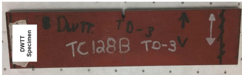
Figure 12: DWTT specimen, transverse orientation (arrow shows rolling direction).
