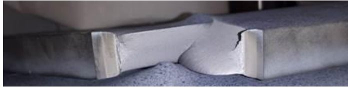
Figure 42: Fracture surface of DWTT specimen tested at intermediate rate
