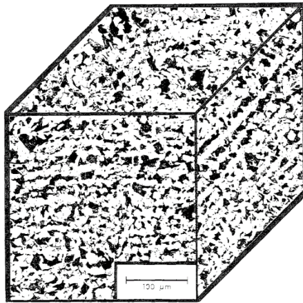
Figure 2: Micrographs of TC128B (the micro-bar in the figure is 100 μm) [34].
