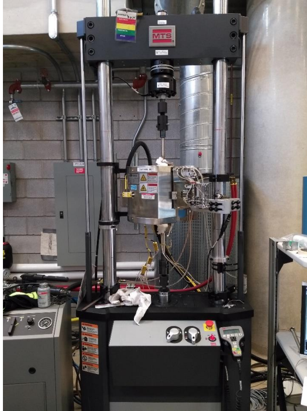
Figure 8: MTS test frame with furnace and extensometer
