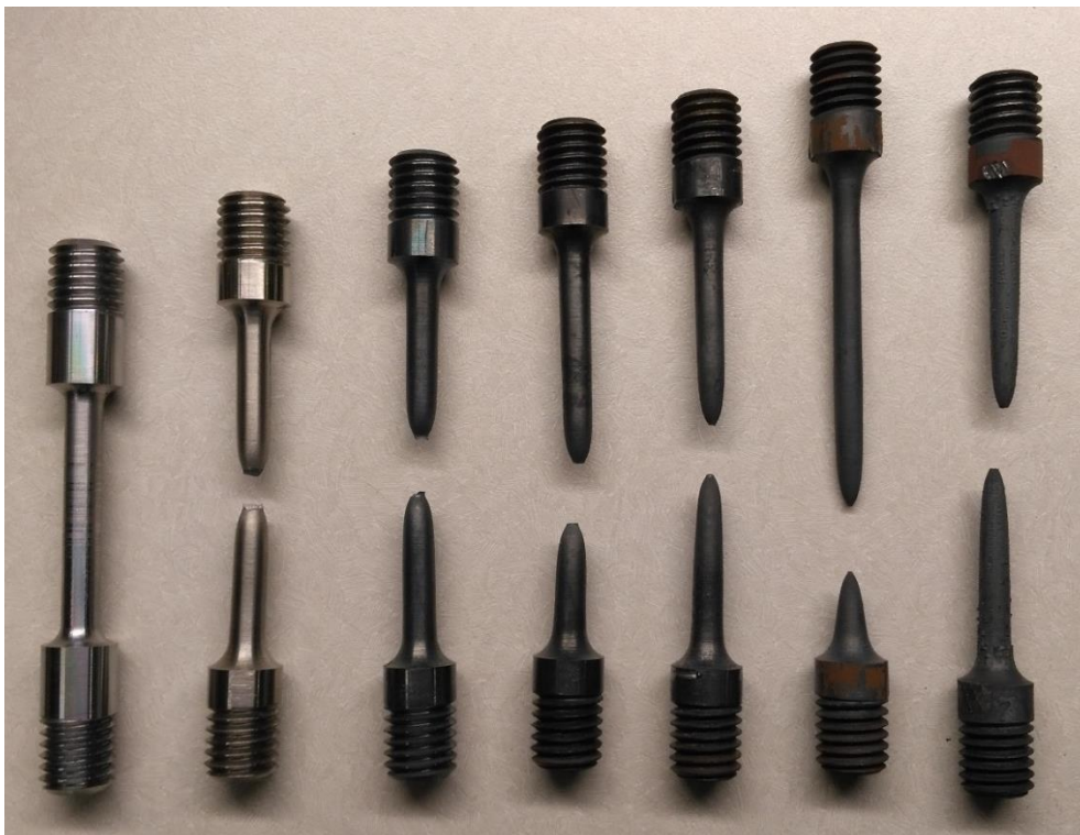
Figure 27: Tensile specimens from left to right; untested, 200°C, 400°C, 500°C, 600°C, 700°C, 800°C.
