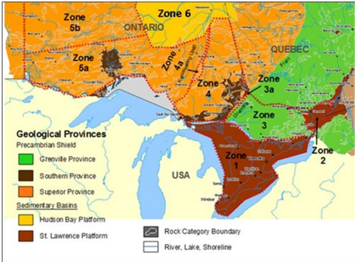
Figure 4.7.1. Detailed Earth resistivity zones of Ontario mapped over Geological Provinces. See OF 8595, Appendix 7 for more details.
