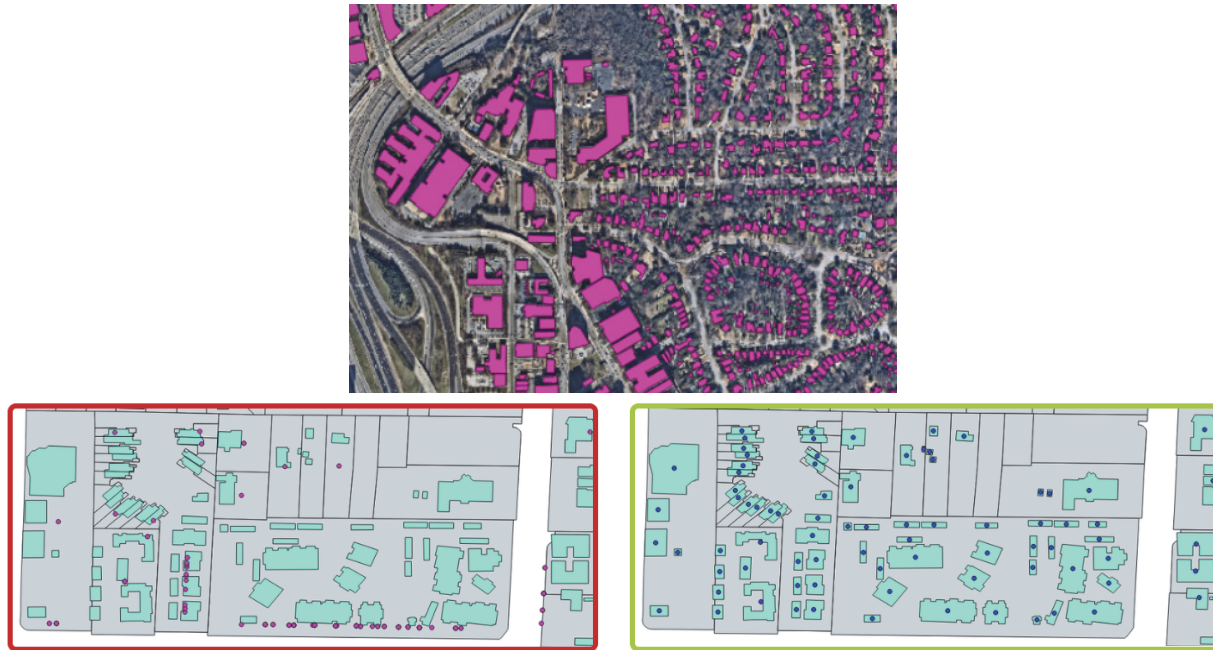
Figure 2 – Example Output from Ecopia's Building Delineation Process
