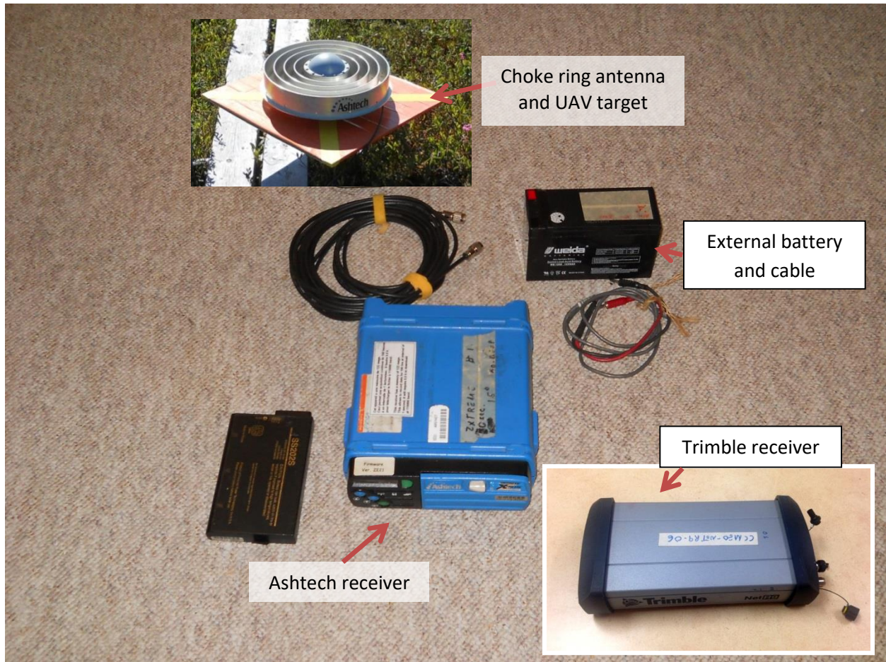
Figure 3.5: GNSS receivers and associated components
