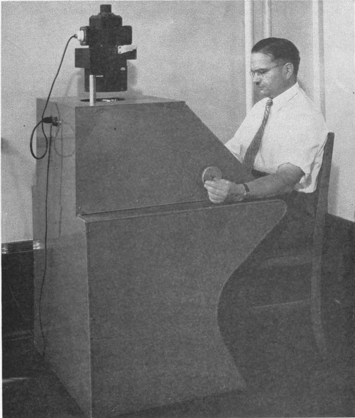
Figure 2.—The new plate measuring engine in operation. A detachable supply cord plugs into a wall outlet, and feeds directly to the toggle switch along side. To the other side of the supply cord is the plug for the mercury vapour lamp in the Omega enlarger head. In order to mount the lamp horizontally in the head, a socket was attached to the back ventilator, and the hole in the top was capped over.
