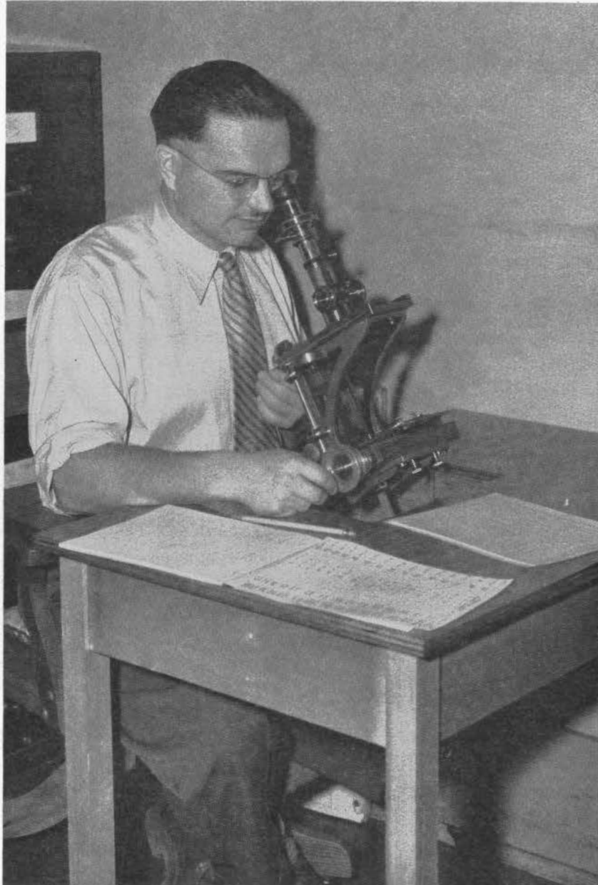
Figure 1.—The Toepfer measuring engine formerly used to scale the PZT plates.
