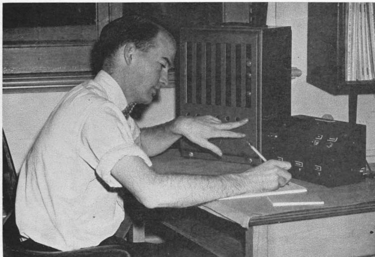
FIG. 8. Controls for the Ottawa P.Z.T. are located in the Time Room. The decade counter measures the fraction of a second between P.Z.T. impulses and second beats of the primary quartz clock. The two switches control the photographic sequence and the fan at the base of the telescope.
