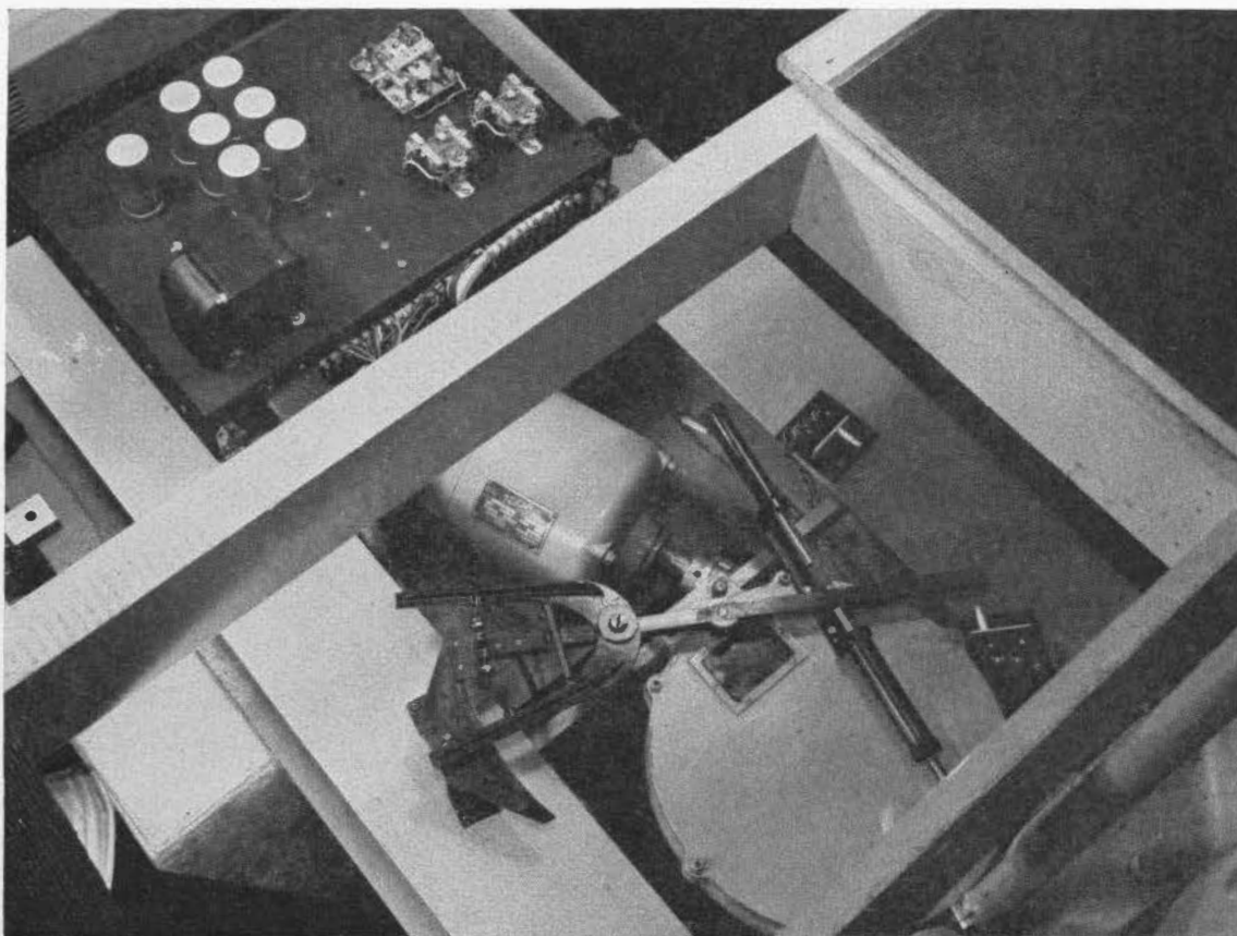
FIG. 4. Ottawa P.Z.T. gear box, reversing motor, and switching mechanism for the automatic reversal of the rotor. An 18-inch boom, driven at its center pin by an arm within the gear box, serves to (a) throw a motor limiting toggle switch with its spring loaded jaws, (b) throw one of two safety switches in case of over run. Spring loaded plungers return the boom to neutral as soon as reversal commences. Also shown is the chassis containing relays, rectifiers and cable terminal strips.
