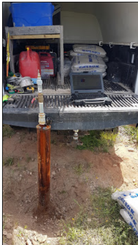
Figure B.26 - Observation well PO-13 before its decommissioning (August 26, 2018)
