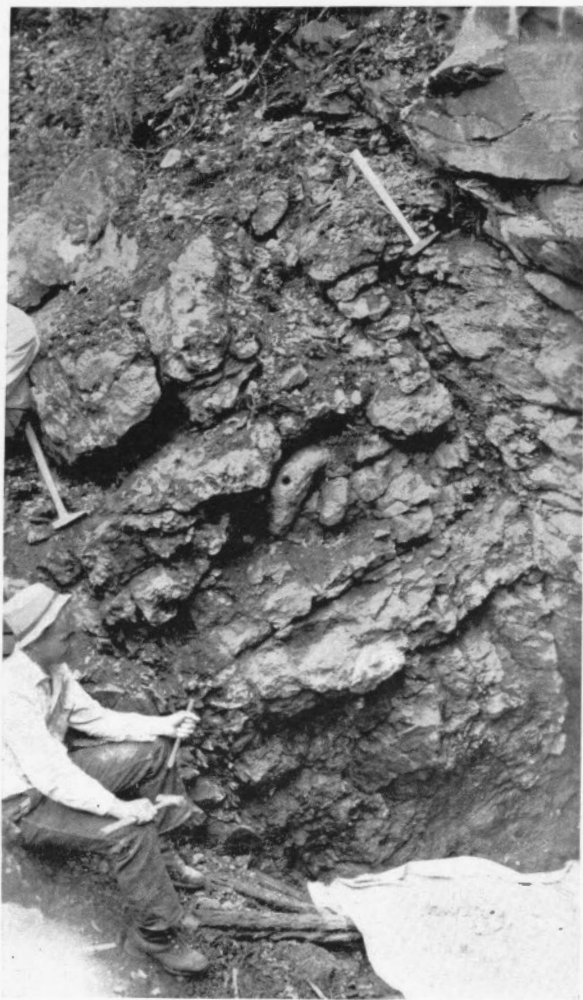
Ore shoot on the No. 1 vein, Silver Standard mine; the width of the shoot is indicated by the distance between the two hammers.
