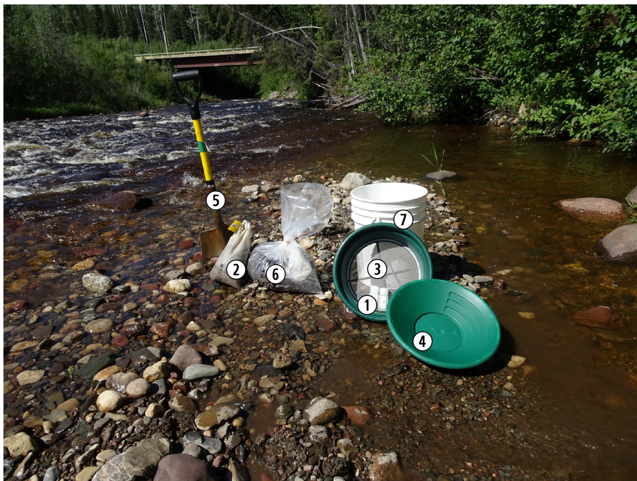
Figure 4.2. Field gear used and samples collected at a typical bulk stream sediment and water sample site located well upstream of human activity. Numbers indicate: 1) two 60 ml water samples (filtered on site with 0.45 \mu\text{m} filter); 2) stream silt sample (~ 2kg wet); 3) #10 mesh (2mm) sieve; 4) pan for washing gravel during sieving; 5) steel shovel; 6) bulk stream sediment (~12 kg of \leq 2\text{mm} sediment); and, 7) bucket that will be lined with pre-labeled sample bag.
