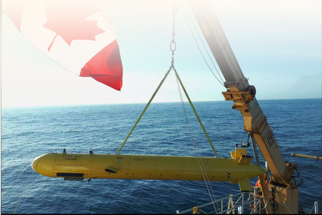
An autonomous underwater vehicle (AUV), is being deployed here as part of a collaborative project with the Government of Nova Scotia to map possible natural oil and gas seeps on the seabed in water depths greater than 2000 metres, offshore NS.
