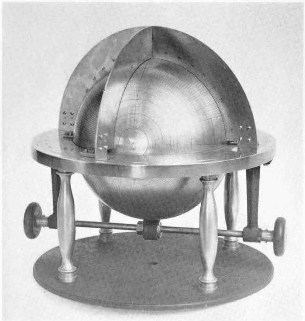
FIG. 24.—Graduated Sphere and Co-ordinate Frame for Heliographic Readings.
