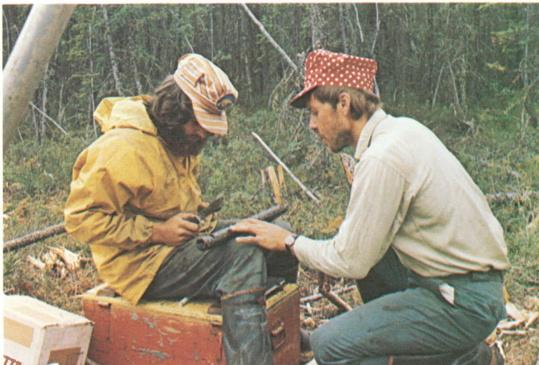
Members of the Geological Survey of Canada inspect core of subsoil obtained in Northwest Territories. Study of soil content and permafrost penetration help scientists determine the capacity of the soil to support engineering and other projects.
