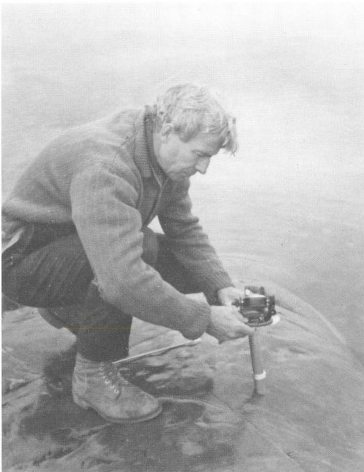
Earth physicist checks the position of a rock core to be used in paleomagnetic survey.
