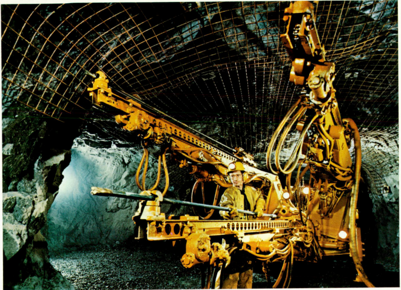
Drill jumbo in use, Sudbury nickel mine.
