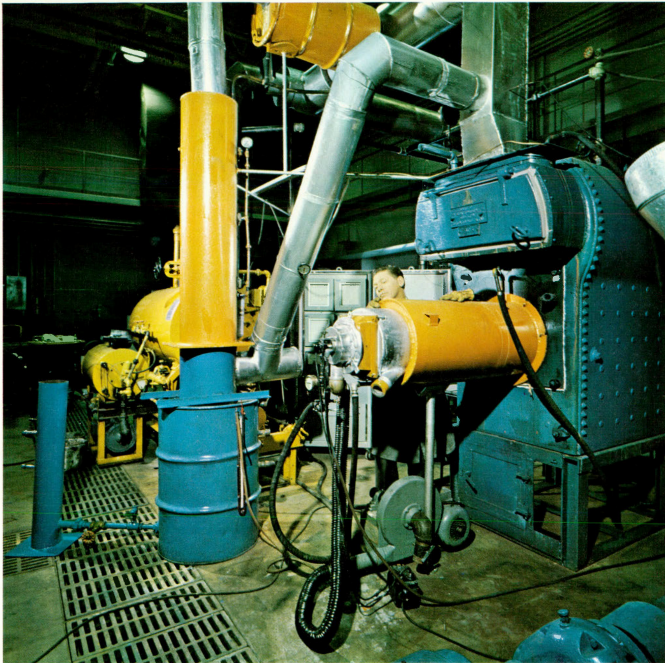
Apparatus for thermal destruction of DDT, Fuels Research Centre, Mines Branch.
