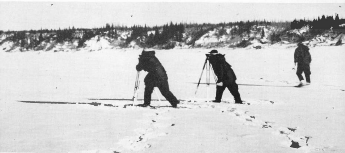
Topographical Survey party extended spirit level control across Labrador in epic winter trek.
