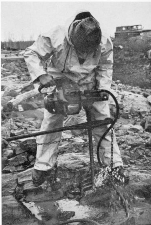
Portable drill is used by geologists to obtain rock core which is to be analyzed for magnetic orientation and structure as part of a micromagnetic study. (G.S.C. 2-2-63)
