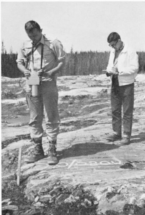
Young master of science candidate attached to geological field party uses new portable fluxgate magnetometer during micromagnetic survey of an iron-ore body. (G.S.C. 1-22-63)
