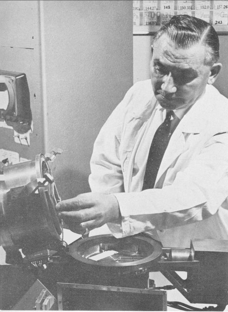
Mines Branch scientist prepares to study an ore sample in the electron probe micro-analyzer for identification and estimation of elements present in the microstructure. (George Hunter #13740)
