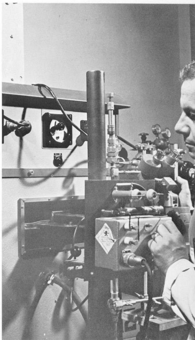
New highly advanced refining apparatus uses narrow band of intense heat, through which metal sample passes, to melt and eliminate impurities, not unlike water being pressed from wet garment that is passed through washing machine wringer. (George Hunter #13742)
