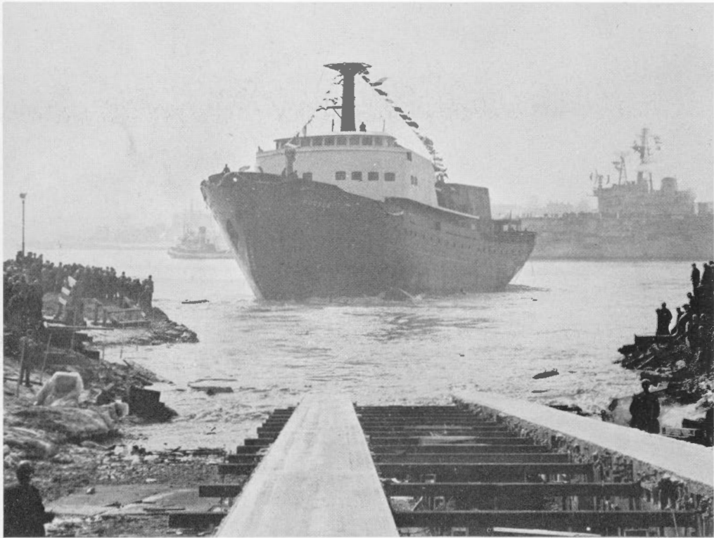
New oceanographic and hydrographic ship, C.S.S. Hudson , was launched in St. John, N.B., in March 1963. The 4,800-ton ship is the Department's largest; it is also the largest vessel in the free world designed for oceanographic research. (M & T S photo)
