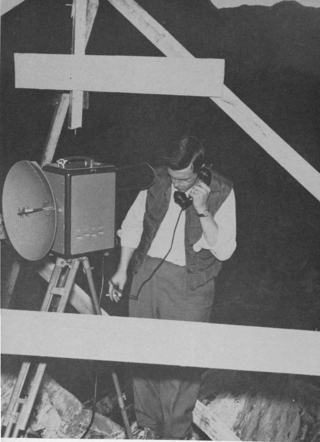
In 1958 the tellurometer, an electronic distance-measuring device of high accuracy, was put to good use in many parts of the country. In hydrographic work it measured distances between survey beacons; in topographical surveys it sometimes replaced slower, more costly triangulation techniques.
