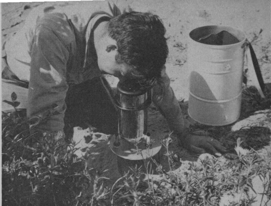
In a study of regional gravity in the region east of Hudson Bay, an Observatory scientist is shown reading a Worden gravimeter near the shore of Clearwater Lake in western New Quebec.
