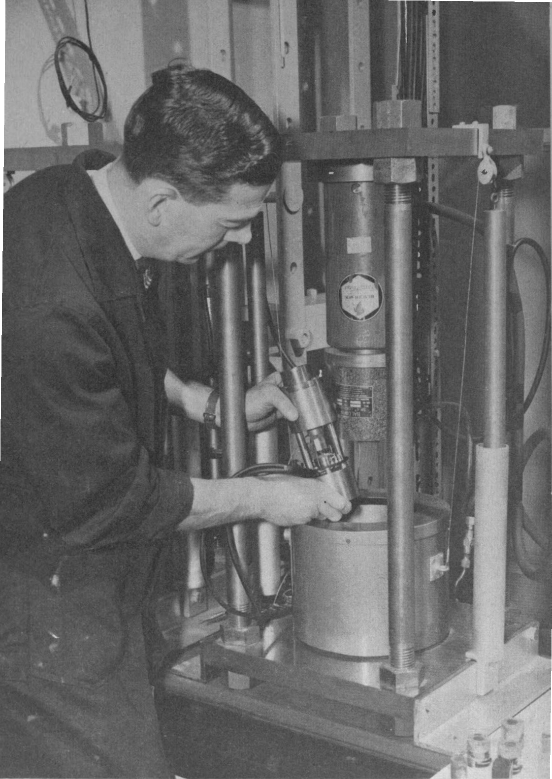
"Bumps" and "outbursts" in certain coal mines in Eastern and Western Canada make mining at depth hazardous and costly. The Branch has under way a long-term project of investigating the complex mechanism of stress relief in mines. Here a Fuels Division engineer studies the strength properties of rock from a coal mine in Nova Scotia.
