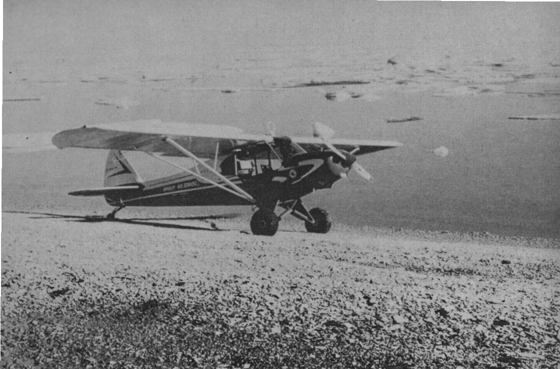
Piper Super Cub used by the Geological Survey of Canada to make landings on rough ground in the Arctic. Specially fitted over-size balloon tires enable the craft to land and take off from rough pebbly surfaces such as shown.
