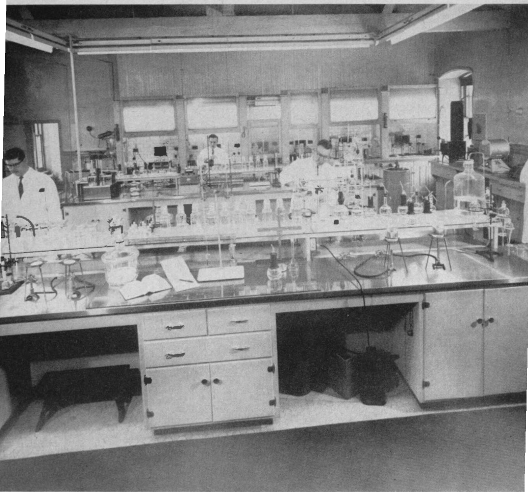
The Survey's rock and mineral analysis laboratory makes detailed chemical analyses of specimens brought in from the field by Survey geologists. Such analyses aid in geological and geochemical interpretation. The laboratory made over 2,700 determinations on samples of rocks, minerals and soils in 1957.
