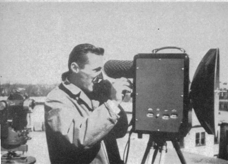
Testing a tellurometer, an electronic distance-measuring device of high accuracy. The instrument was put to work in the Ungava Peninsula, in Northwest Territories and on the Prairies with great savings both in time and cost.
