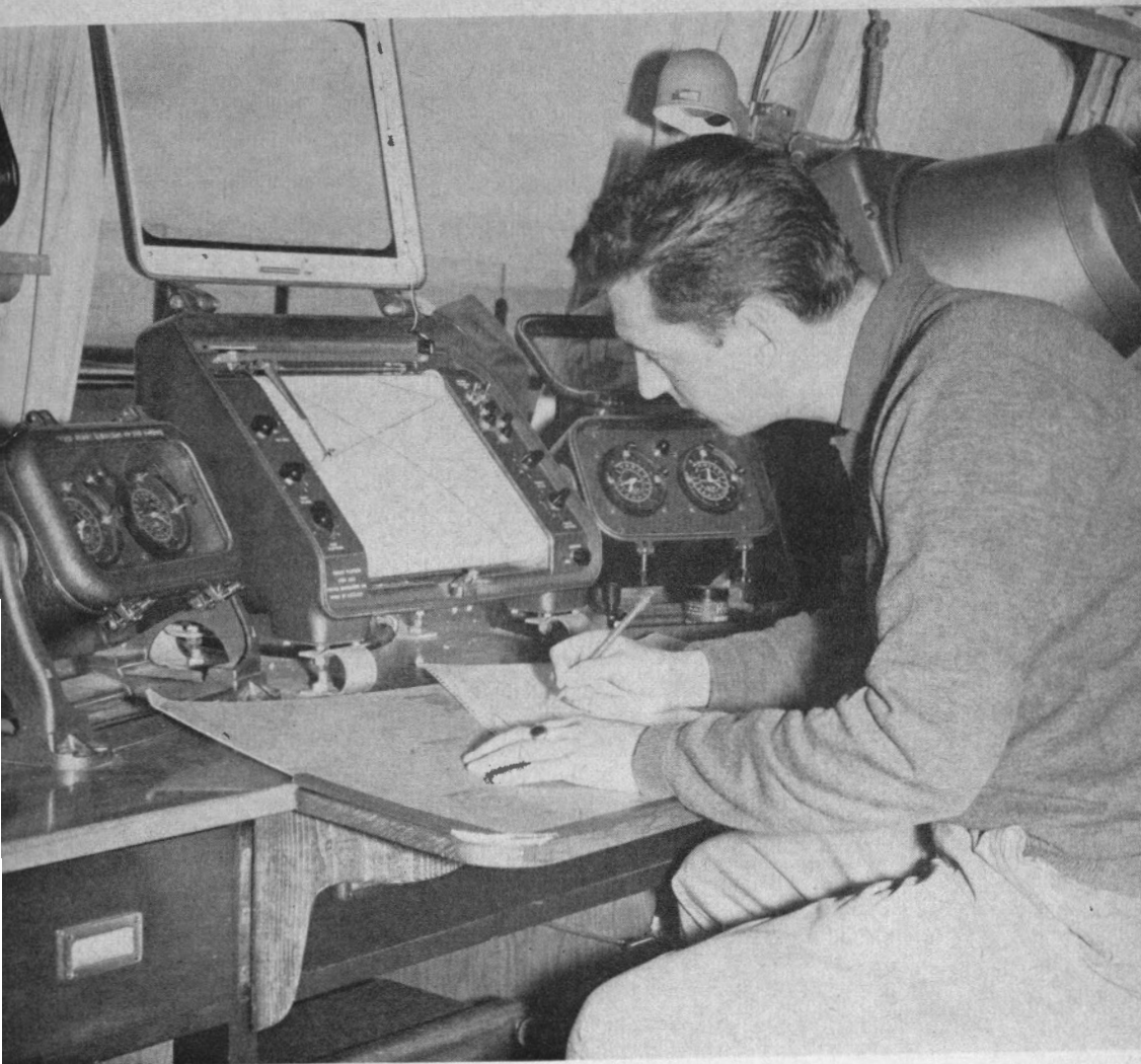
A hydrographer aboard the Baffin records the ship's position as shown by two-range Decca equipment. The Decometer readings give the precise position of the ship while the log provides a continuous graphical record of her course.
