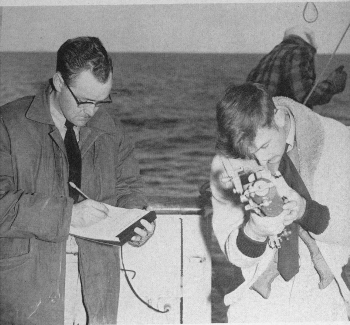
Reading a reversing deep-sea thermometer after the completion of an oceanographic station. This involves determining the temperature and obtaining a sample of sea water from depths of 10, 20, 30, 50, 75 and 100 meters.
