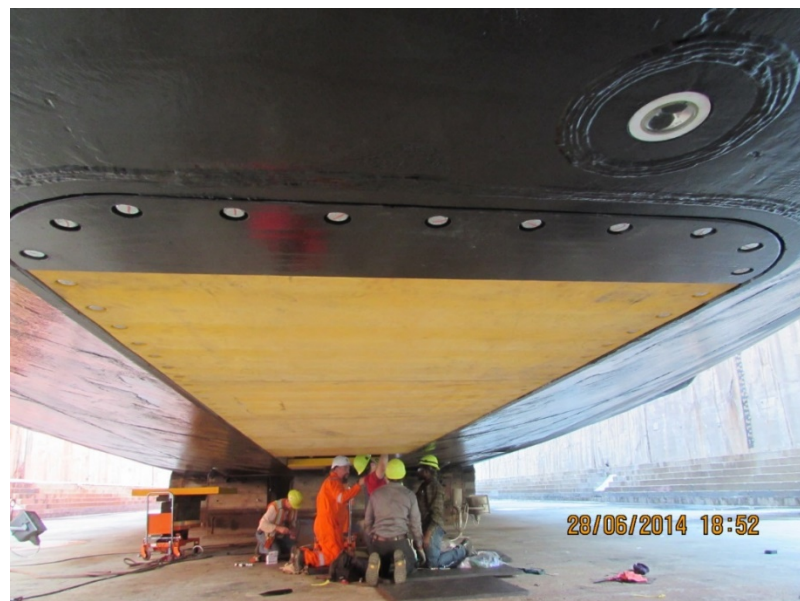
Figure 2.3. Installation of the EM122 multibeam system on the hull of the CCGS Louis S. St-Laurent.
