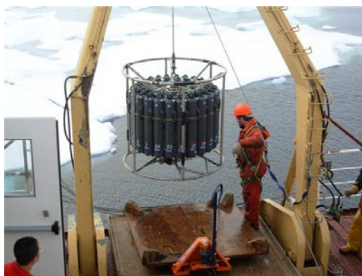
Figure 4.2. The 24-bottle rosette with the SBE9+ CTD is deployed from the mid-ships A-frame (photo 2008).
