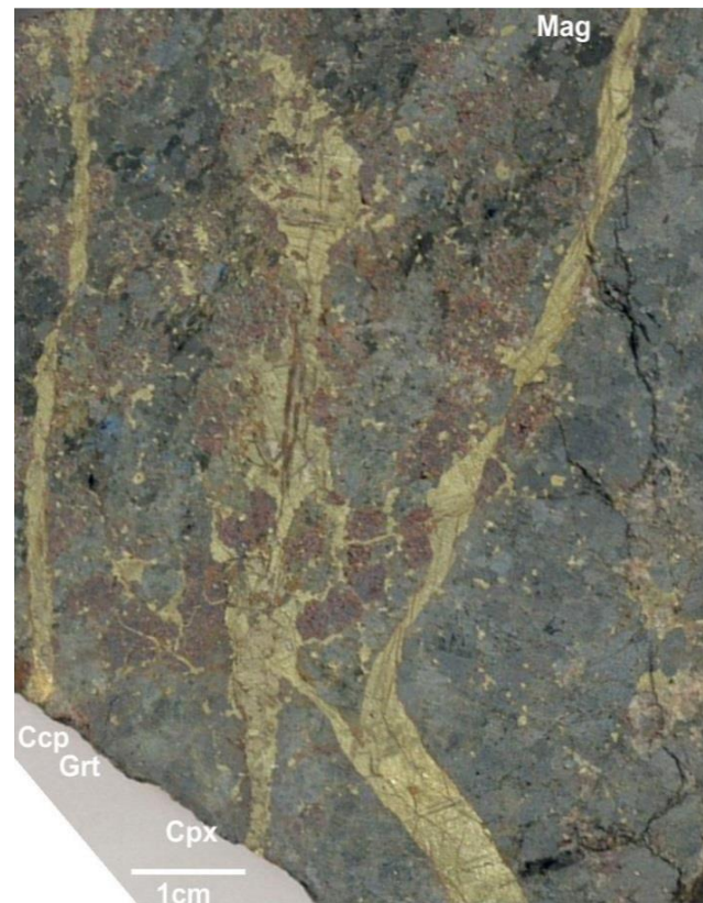
Figure 6.23. Bing showing calc-silicate rock with clinopyroxene, garnet and magnetite veined by chalcopyrite. Such veins are interpreted as remobilization of sulphides after peak metamorphism. Photo courtesy of Richmond Minerals from Antonoff et al. (2007).
