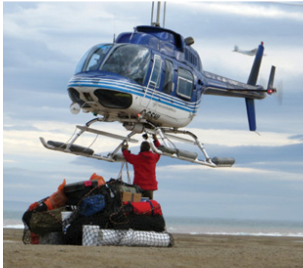
A sling load is attached to a helicopter on Banks Island, Northwest Territories.
