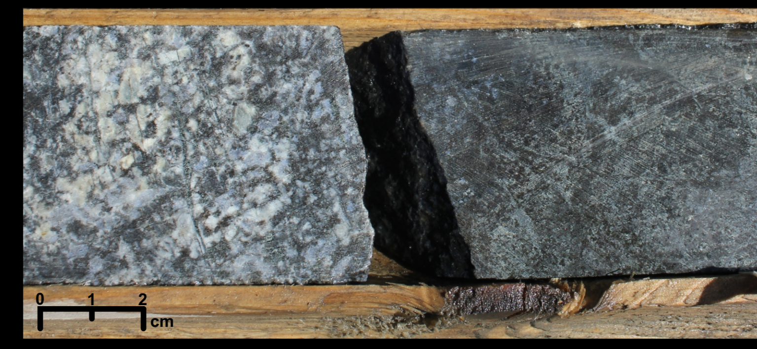
Fig. 3. Sharp primary intrusive contact between granodiorite (left) and serpenitized peridotite (right) with preserved medium grained cumulate texture (pseudomorph pyroxene and olivine). Drillhole FW-08-06 at 103.51 m.
