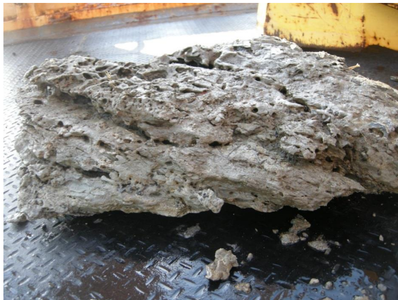
Figure 16. Carbonate crust on ships deck
