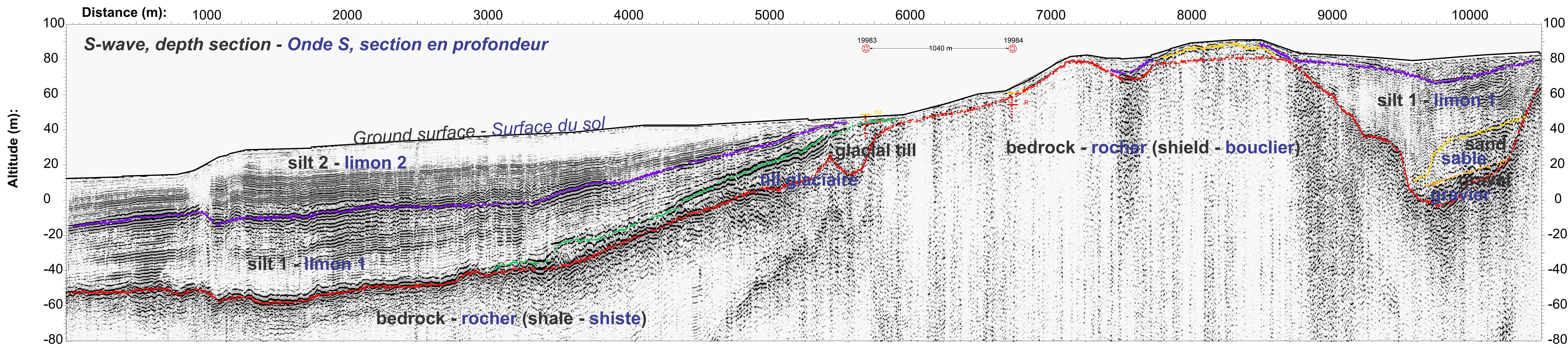
Shear-wave seismic section showing extremely high resolution. This geophysical method is being developed at the GSC using innovative landstreamer technology. Shear-wave properties are essential for mapping potential landslides and earthquake soil
