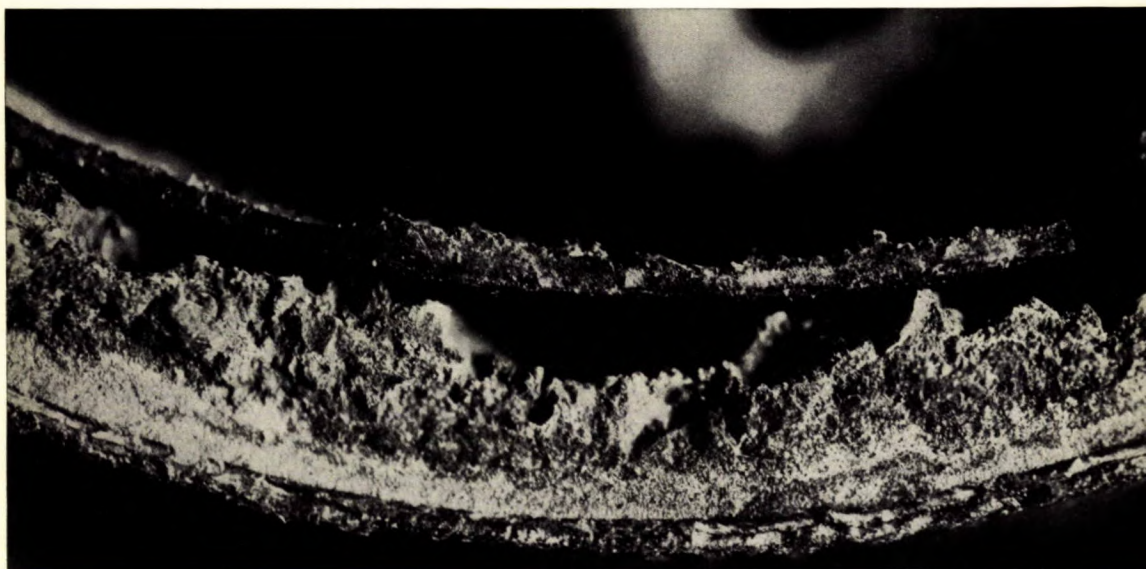
Figure 56. Scale build-up on Type 446 tube (x16) after 481 hours and 869 hours (typical cross-sections of scale; scale removed about 15 inches from tube insert).
