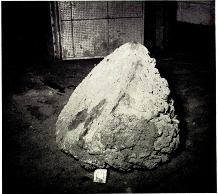
Figure 51b. Slag accumulation from target after a 247-hour test.
