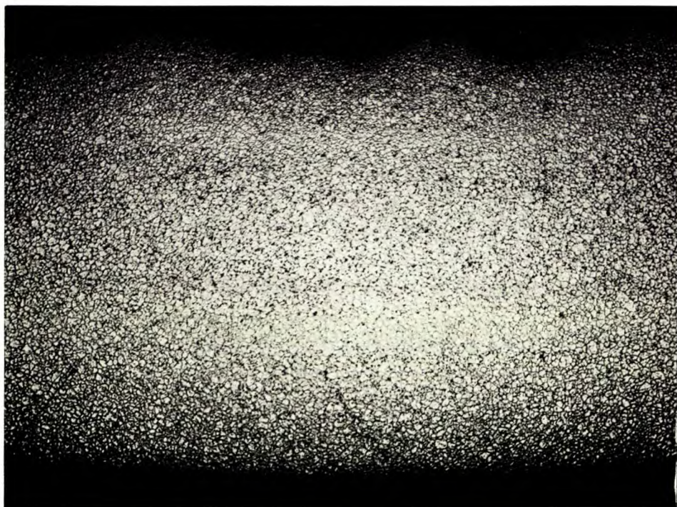
Figure 60b. Corrosion attack on Type 309 (row 12, tube 6 (x50), 1 inch from ceramic insert).
