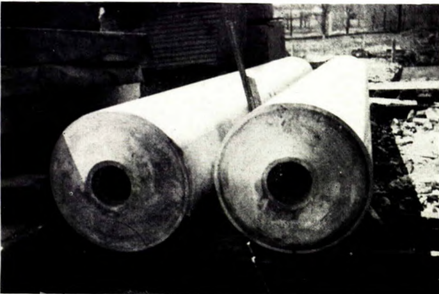
(d) Finished blocks ready for mounting on steel shaft.
