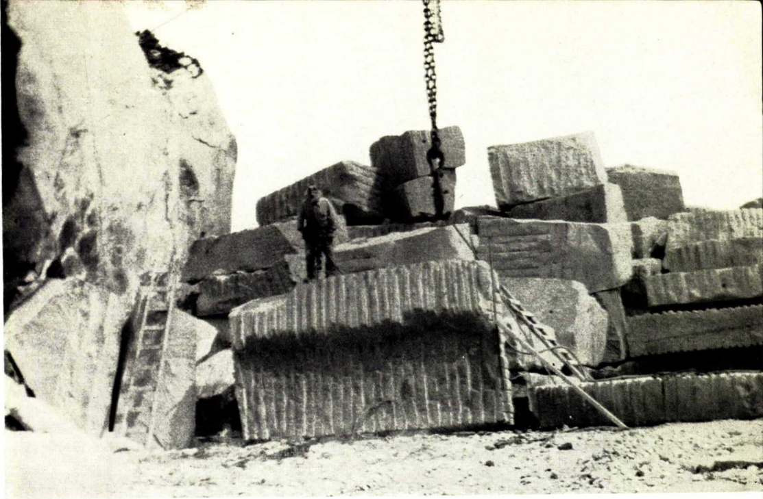
Figure 42 | J. A. & C. H. McDonald Limited quarry, Haddington Island, B.C. This block measures 15 ft. long, 7½ ft. high and 2 ft. wide and was quarried for the new Bank of Commerce Building, Vancouver, B.C.
