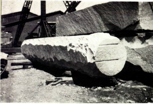
(a) Rough blocks in plant yard at Iberville, Que., partly shaped by hand.
