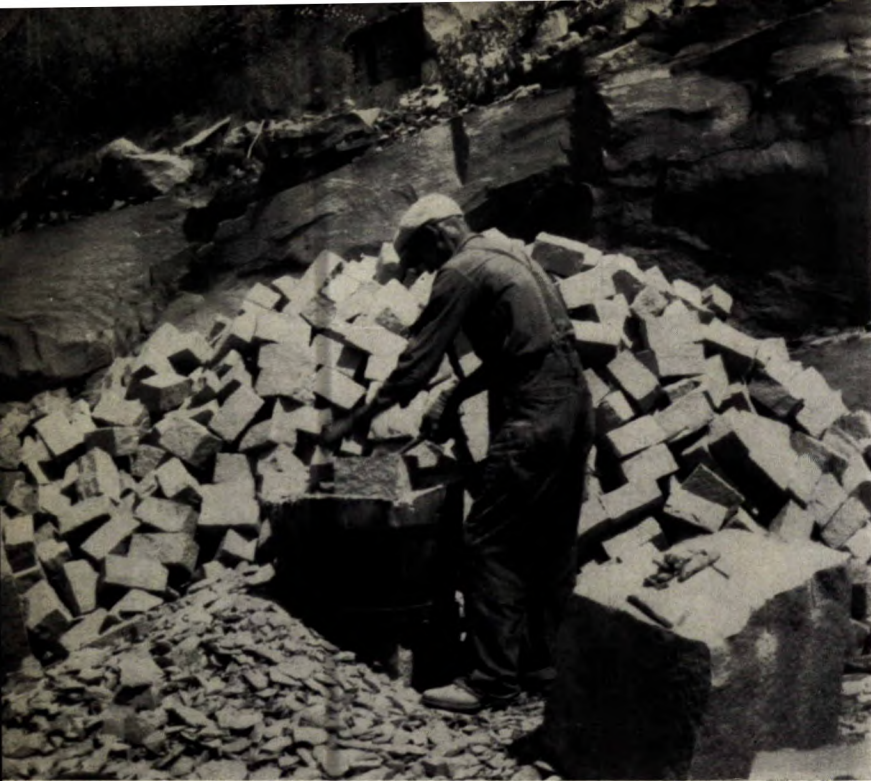
Figure 17 | Brodie's Limited quarry, Guenette District, Que. Paving block cutter at work with pile of finished blocks.
