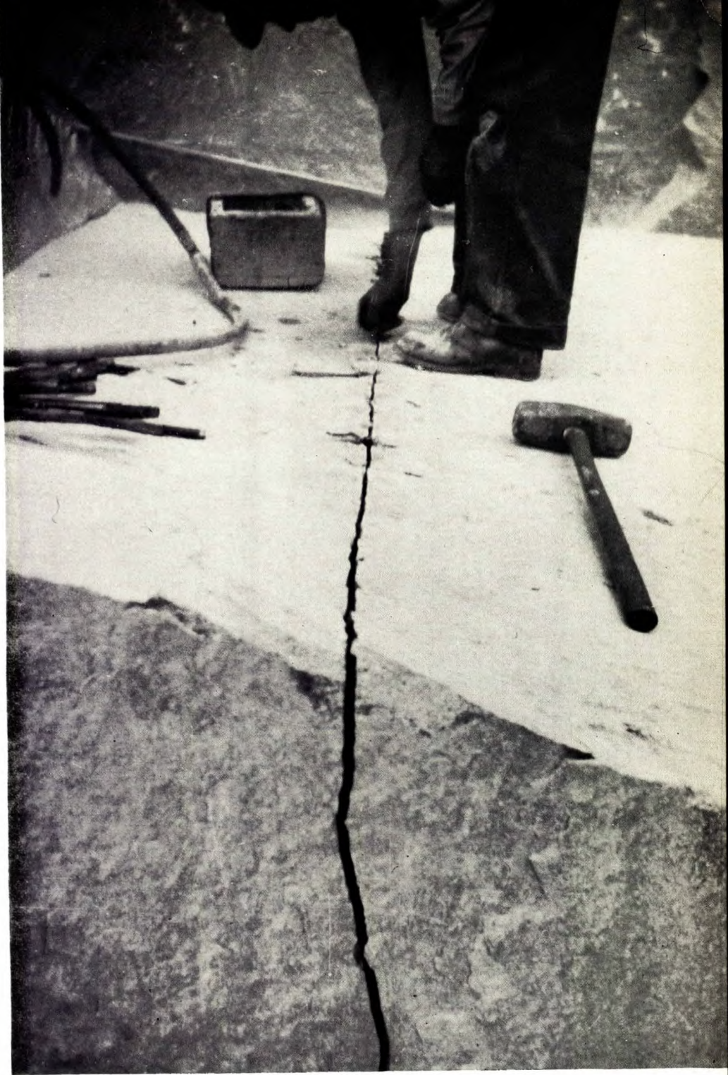
Figure 16 | Splitting granite by means of 'plug and feather' at Atlas Granite Company, Limited, quarry, Guenette District, Que.
