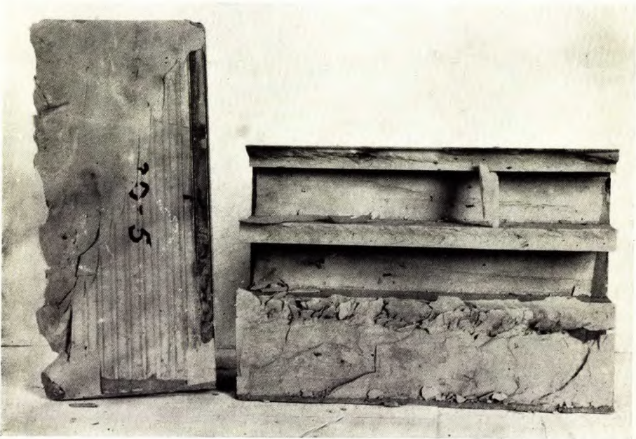
B. Compressive strength: failure due to shear.
