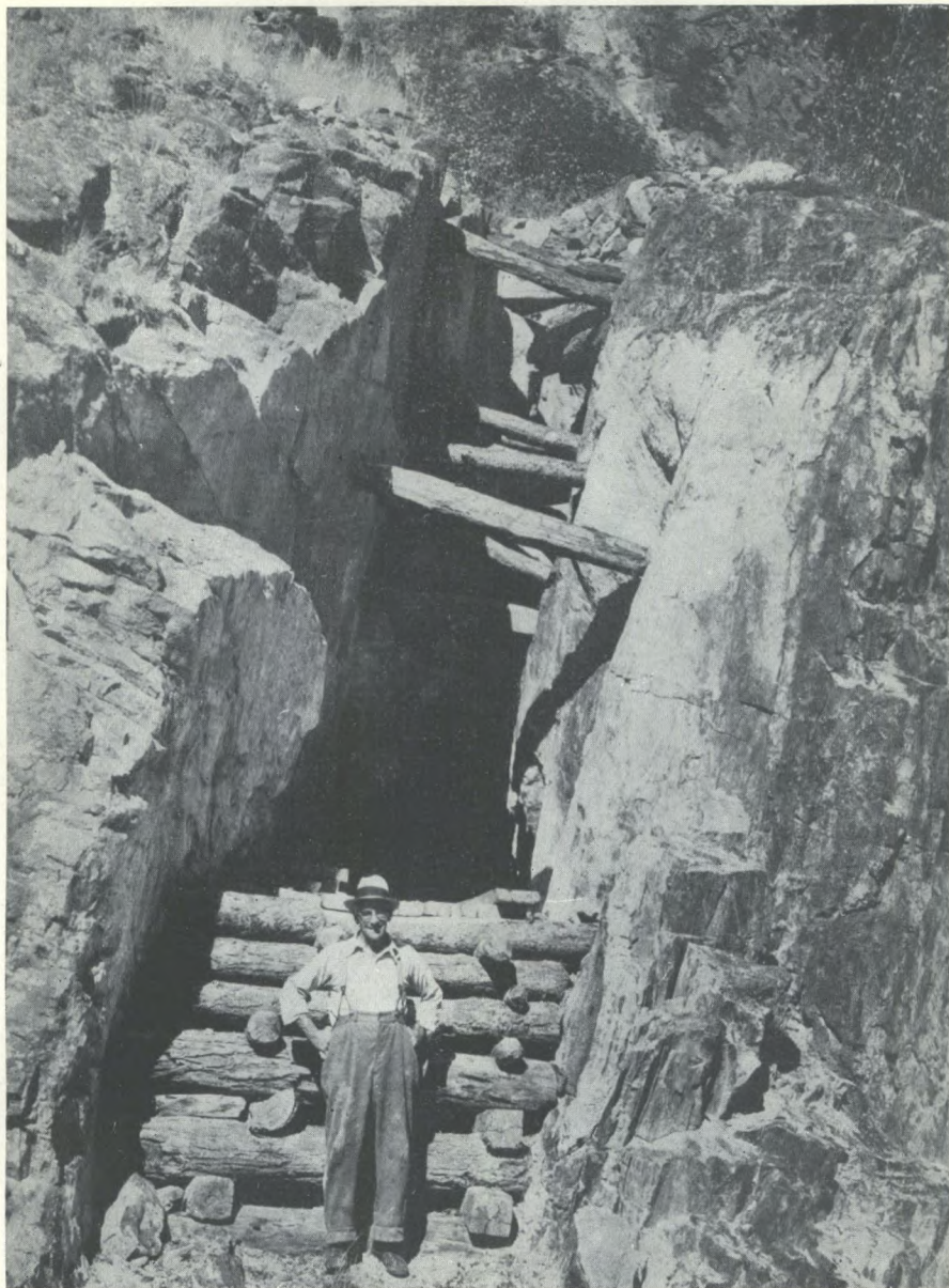
Talc working on Lake Shore claim, mile 90, Pacific Great Eastern Railway, near McGillivray, Lillooet Mining Division, B.C. The talc body occupies a sheared zone in an assemblage of serpentinized greenstones and chloritized slates. It illustrates well the typical association and mode of origin of a talc deposit by hydrothermal alteration of an ultrabasic rock—probably upon a fault-plane, which provided the channel for circulating hot waters. (See page 55)
