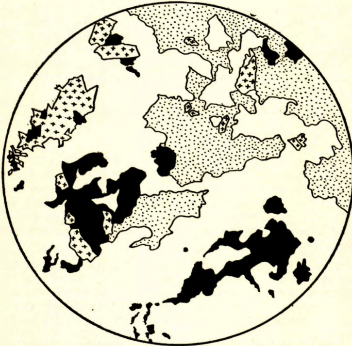
Figure 1. Drawing of polished section of gold ore from Negus Gold Mines, Limited, Yellowknife, N.W.T. Gold—black; jamesonite—dotted; arsenopyrite—crossed; quartz—plain white. Magnification: X 20 approximately.
