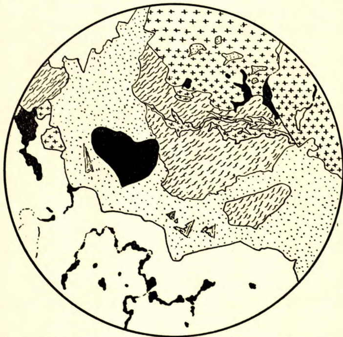
Figure 1. Drawing of polished section of gold ore from Camlaren Mines, Yellowknife, N.W.T. Pyrite—crossed; galena—dotted; pyrrhotite—waved lines; gold—black; gangue—white. Magnification: X 50 approximately.
