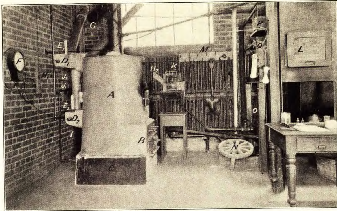
Domestic furnace and auxiliary test apparatus. (Water meter; and radiation, expansion, and water service tanks not shown.) A. Domestic hot-water boiler. B. Ordinary ash-pit. C. False ash-pit into which fuel is dumped for quenching. D 1 , D 2 . Flow and return headers. E 1 , E 2 . Thermometers in flow and return headers. F. Thermograph recording flow and return water temperatures. G. Flue-pipe entering chimney. H 1 , H 2 . Draught adjustments on butterfly and flap dampers in flue-pipe. I. Draught recorder measuring over-fire draught. J 1 , J 2 . Draught gauges measuring over-fire and flue-pipe draughts. K. Flue gas sampling and analysing equipment. L. Recording pyrometer measuring flue gas temperatures. M. Fire tool rack. N. Wheel-type gas burner for igniting fuels. O. Gas meter measuring gas supplied for ignition. P. Hygrograph recording indoor humidity. Q. Thermograph recording indoor and outdoor temperatures.
