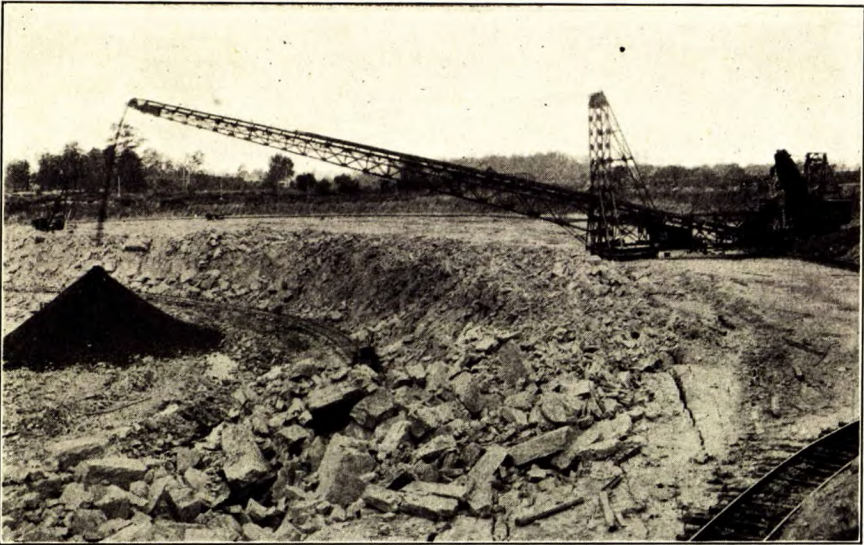
Courtesy: Greenville Mfg. Works, Greenville, Ohio. Machine applicable to the placement of overburden.
