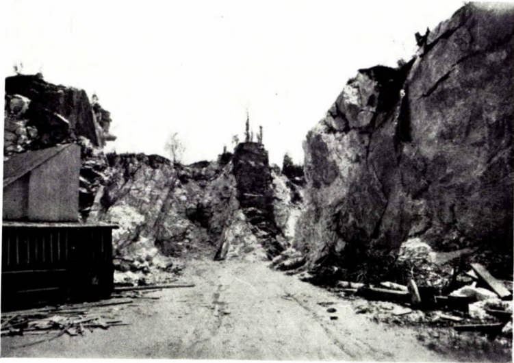
A. "White" quarry of Randolph and Baker, Ltd., Green Head Island, St. John County, N.B. The vertical band of dark rock in the centre of the illustration is a dyke of trap rock.
