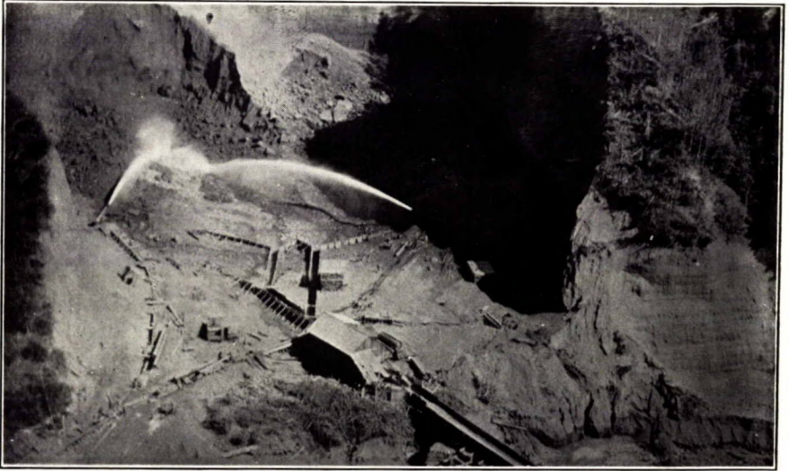
A. Hydraulic mining gold-bearing gravels, Cariboo area, B.C.
