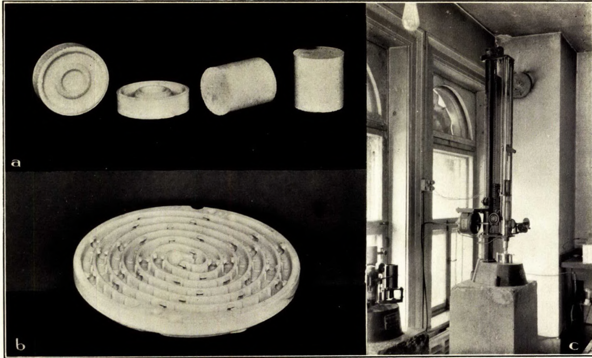
a. Test pieces. b. Typical electric stove-plate. c. Page impact testing machine.
