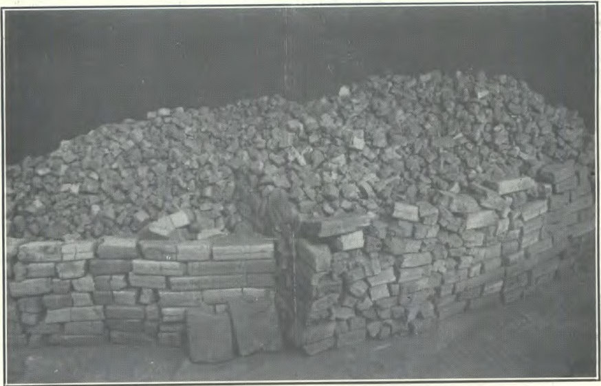
B. Low-temperature carbonization coke by Illingworth process as sold on English market
