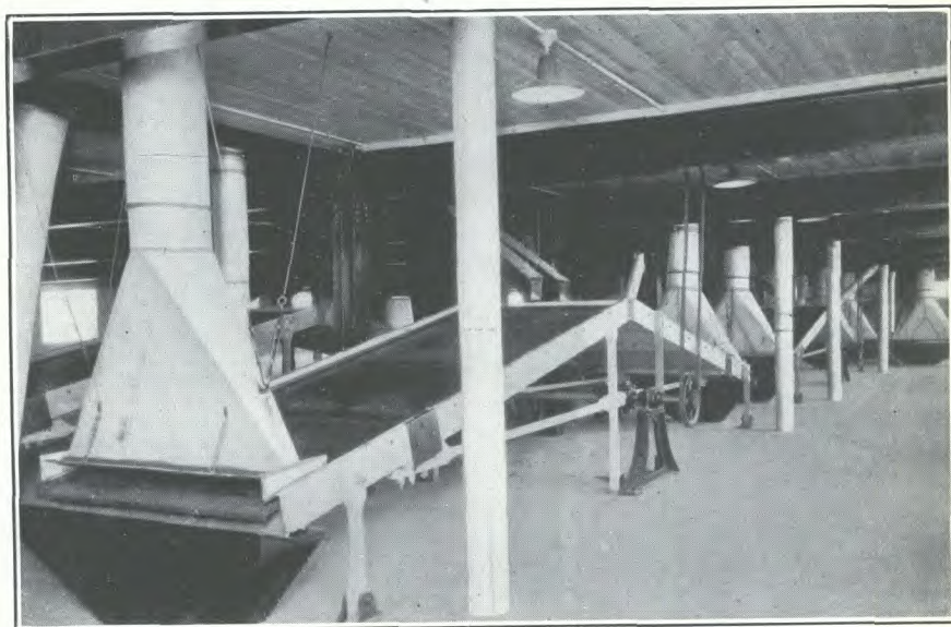
B. Shaking screens conveying asbestos fibre to suction apparatus, separating and sizing, Johnson's mill, Thetford mines, Quebec. (Photos by courtesy of Johnson's Company)
