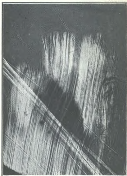
D. Black Lake fibre fracture. \times 350 .
