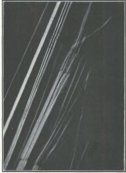
B. Break in fibre from Pilbarra district, Western Australia. \times 150 .
