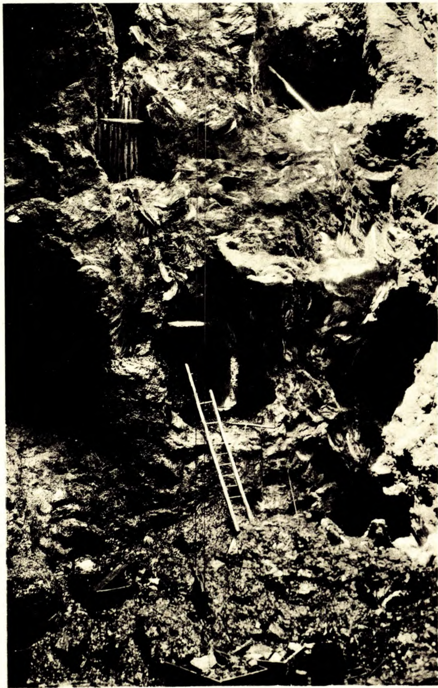
view taken at the bottom of main pit (see Plate XIVA) at Lacey mine, concession VII, lot 11, Loughborough township, Ont., showing principal mica lead. The vertical vein extends across almost the entire width of the face shown, and mica is now won by caving of the old stopes and drifts
