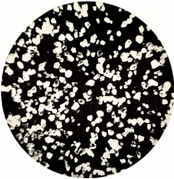
A. Photomicrograph of finer grained aggregate from Alberta bituminous sand. (Magnification: x 22.)
