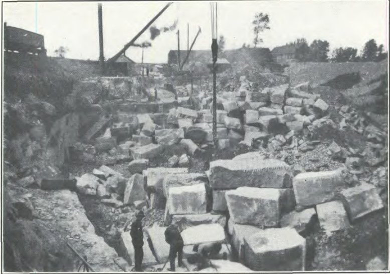
A. Lockport dolomite. Heavily bedded stone (Gasport) at the base of the formation, Queenston Quarry Co., Ltd., St. David, Lincoln county.
