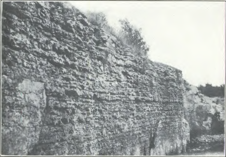
A. Cherty Onondaga limestone, Buel quarry, near Windmill Point, Welland county. The chert resists weathering action and forms projections on a weathered surface.
