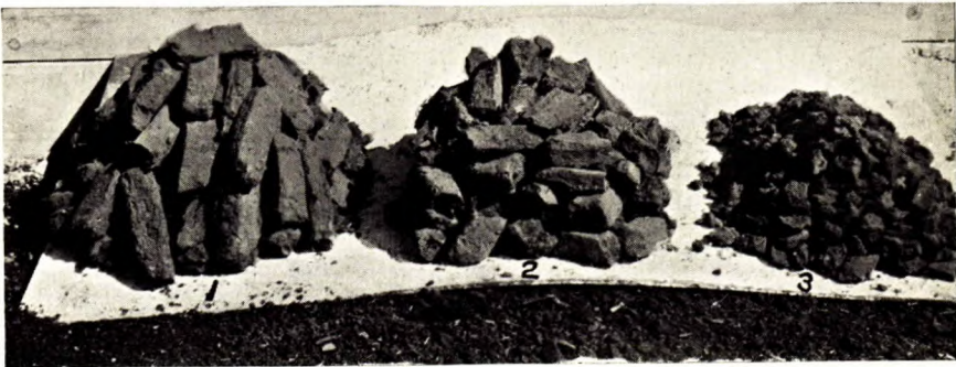
Air-dried peat and peat charcoal:— (1) Large size (machine-made) briquettes (2) Peat, broken pieces, as carbonized (3) Peat charcoal produced
