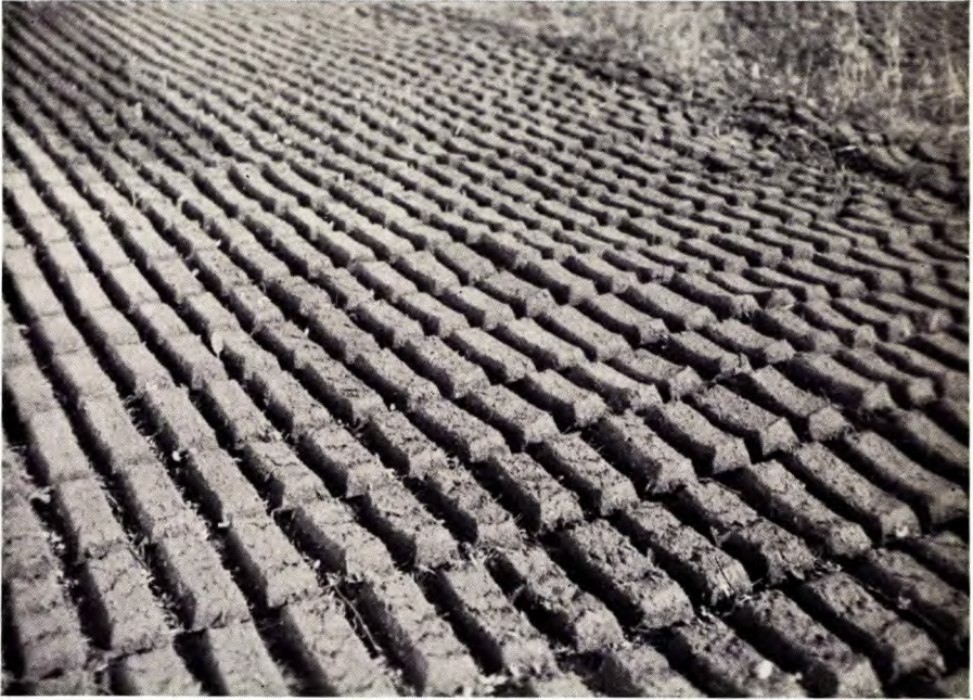
Peat spread on the field, at Alfred, as it appears when partly dry
