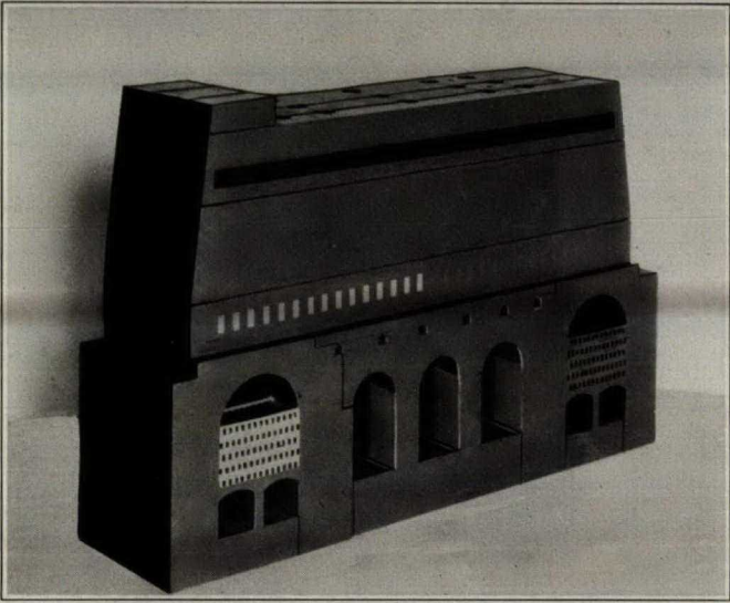
A. Model, Otto-Hoffman oven, vertical section through coking chamber and omnibus regenerators.
