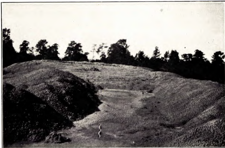
Outcrop of bentonite bed at Clay Spur, near Newcastle, Wyoming. The deposit is flat-lying and has little or no overburden. The photograph shows the bed partly broken up and the clay stock-piled. The peculiar weathering crust exhibited by bentonite is shown.
