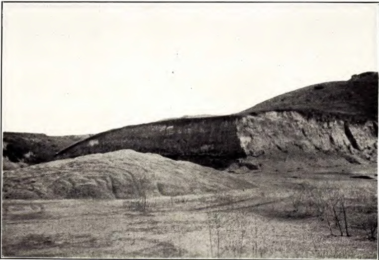
Bentonite-like clay (otaylite), possibly a sub-variety of montmorillonite or leverrierite, near Olay, south of San Diego, California. The clay forms a bed, 5 feet thick, at the base of the bank, and is overlain by sand. It is, variously, pink, white and brown, and is used for oil refining. Stock pile in the middle foreground.
