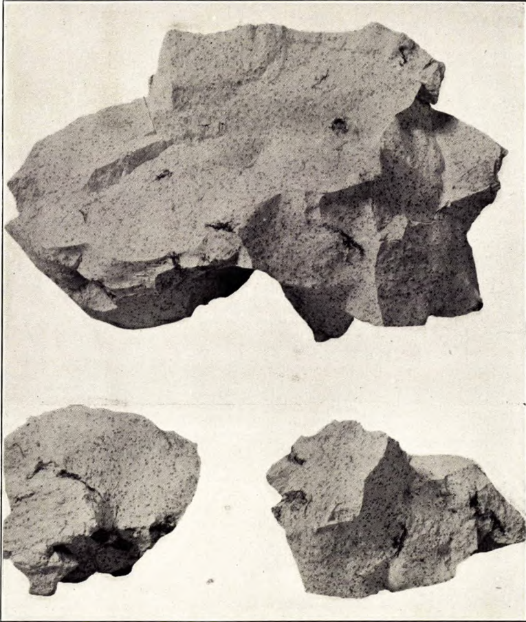
Bentonite from mine of the Rosedale Coal Company, Rosedale, Alberta. This clay forms a thin parting between two coal seams. It is hard and dense, has a drab, grey colour and contains carbonaceous material. In colloidal character, it compares well with the Wyoming bentonite.
