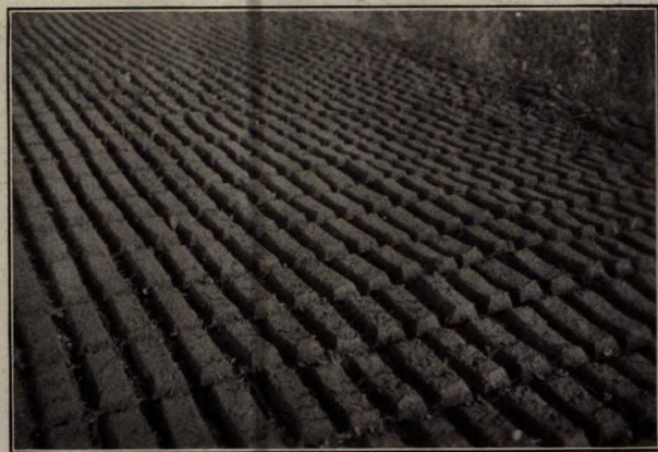
Peat fuel laid on the field. This plate shows very clearly the effect of the improved longitudinal and cross cutters
