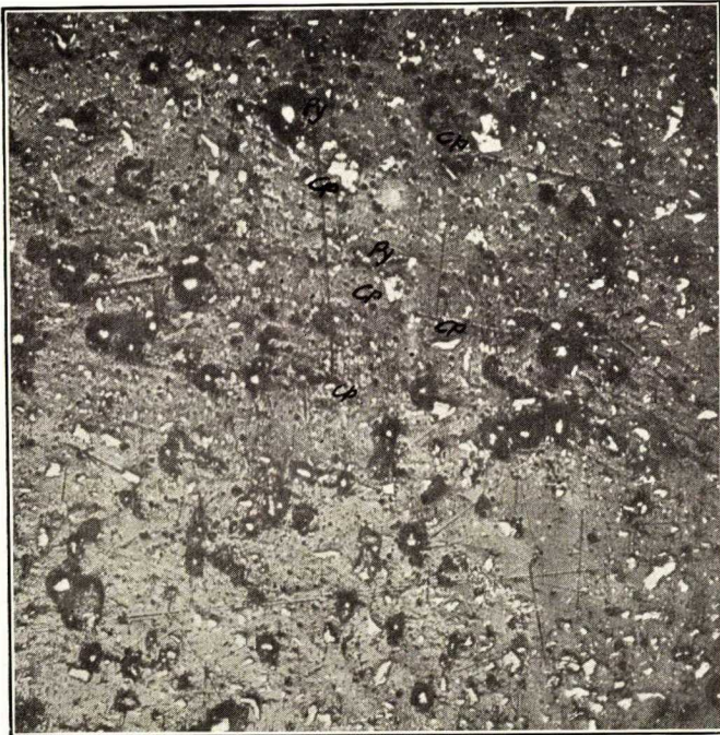
Copper concentrate from Flin Flon sulphide ore, x 100
