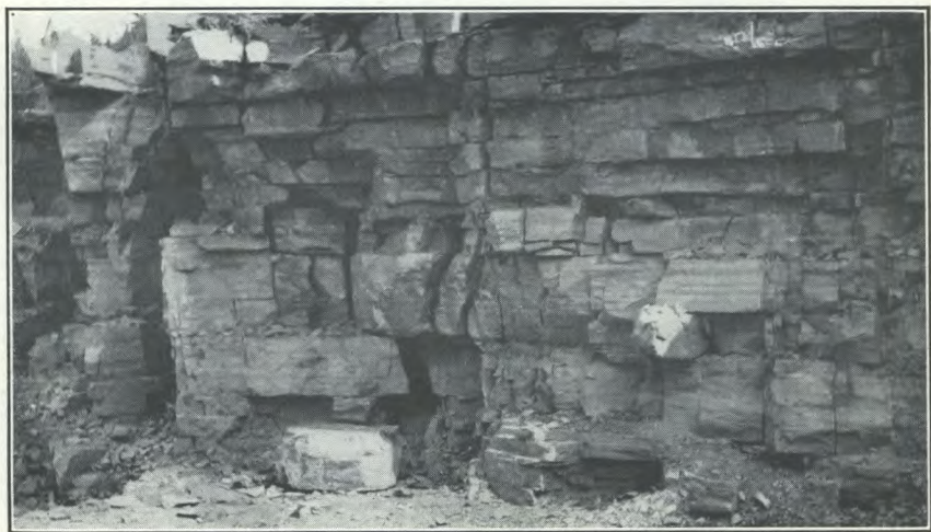
Beds of Beekmantown dolomite in Laberge quarry near Chateauguay, Que. Used for road material on Woodlands-Chateauguay road. Road material sample No. 257
