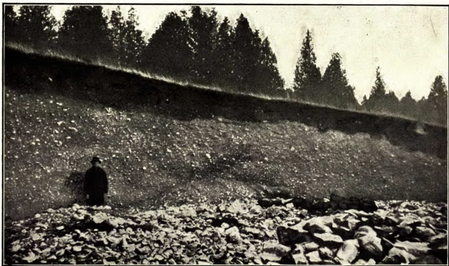
Pit No. 50 (Murphy's). The gravel turns more bouldery and less markedly stratified towards the top of the deposit (left of picture).
